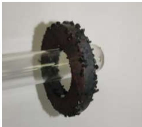
Fig. 1. The iron- Impregnated charcoal particles are attracted to the magnet, indicating the success of the production process
