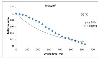
**Fig5.** Determination of the drying constant; (k) of Lewis's equation at the maximum radiation intensity of 1000 and 900 W/m2 and different drying air temperature levels.
