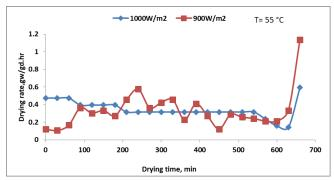
**Fig3.** The influence of infra-red radiation intensity and drying air temperature on tomato leathers drying rate at drying air velocity 0.5 m/s and thickness of samples 0.8 cm. on tomato leathers drying rate.
