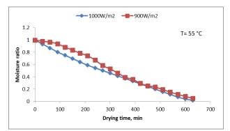
**Fig4**.Tomatoes leathers moisture ratio as related to drying time at different levels of infrared radiation and different drying air temperature.
