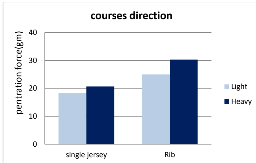
Fig. 3. Relation between the penetration force in courses direction with fabric structure at the two levels of fabric weight (light and heavy).
