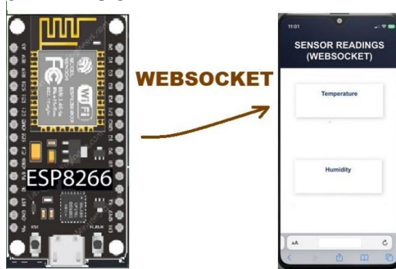
Figure 12 websocket for exchange data between ESP8266 and web or mobile app.
