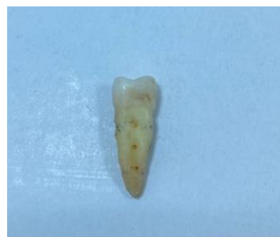
Figure (1): Tooth Sample with indentations made on root surface at 3, 5, 7 mm from the apex.
