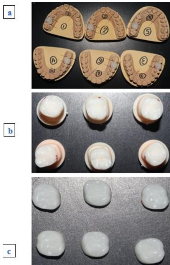
Figure (7): PMMA milled crowns; (a) PMMA crowns fabricated on stone dies, (b) PMMA crowns fabricated on 3D printed dies, (c) PMMA crowns fabricated on virtual dies.
