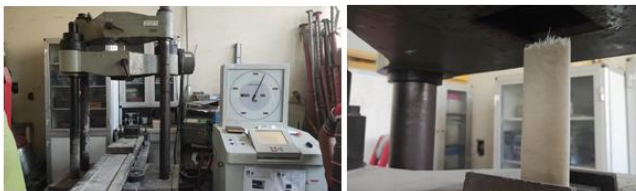
Fig 10. Tension test for GFRP specimens
