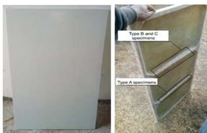
Fig 5. Timber-GFRP panel after fabrication and painting
