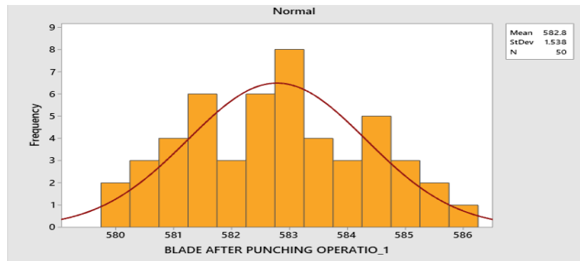
Fig. 8 Histogram of weight of blades after punching process
