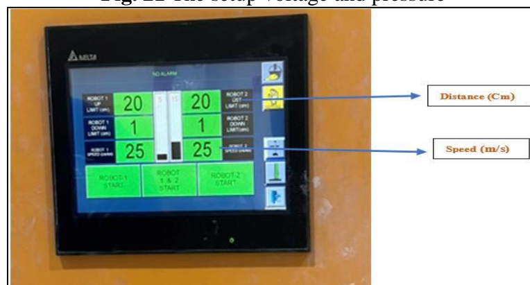
Fig. 22 The setup of the distance and speed
