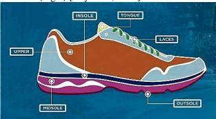
Fig. 2. Different components of sports footwear [Roy et al, 2023].
