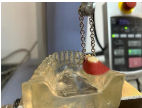
Figure (3) showing the pulling action of the testing machine
