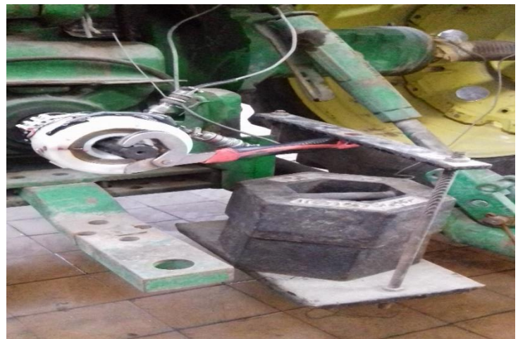
Figure (6). A platform for static calibration of the torque for the fabricated torque sensor.
