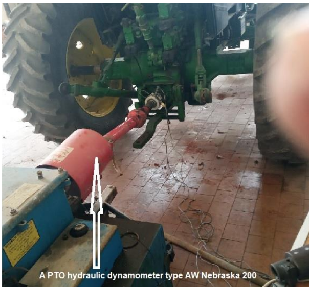
Figure (7). The load produced by the AW PTO hydraulic dynamometer was stately by an interface commercial PTO torque meter and by the fabricated PTO torque transducer.
