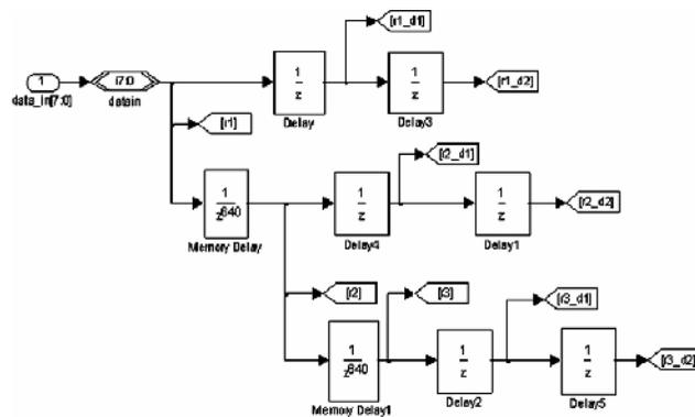
**Figure (3):** Line buffer principle for a 2D FIR filter for a 640x480 frame.
