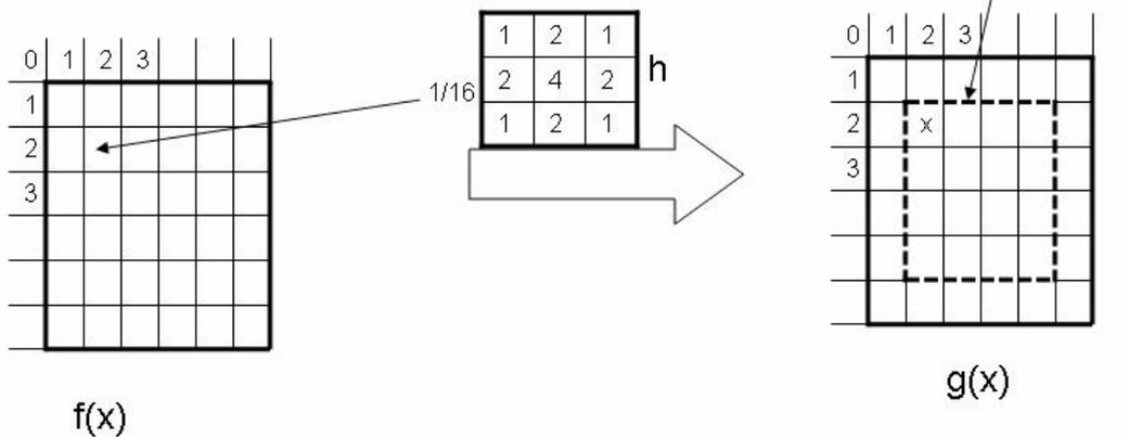
**Figure (1):** Gaussian pyramid filter kernel
