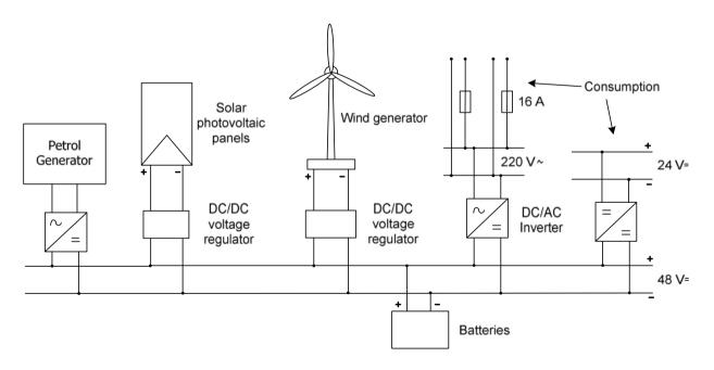
Figure (2): Simplified scheme of mobile hybrid power system
