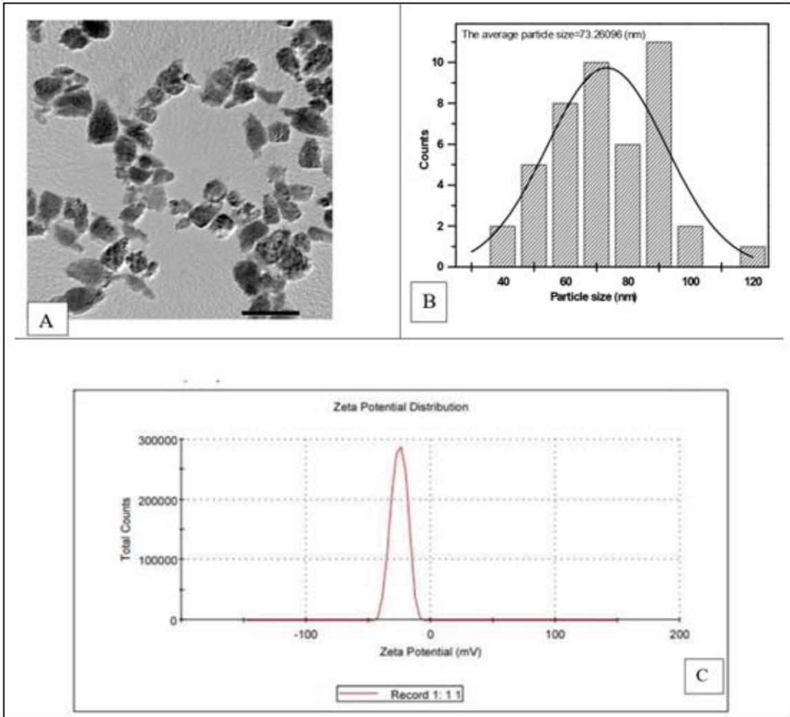
**Fig.1.** Characterization of CUR-NPS; (A): TEM micrograph; (B): Histogram of the average particles size; (C): Zeta potential histogram.
