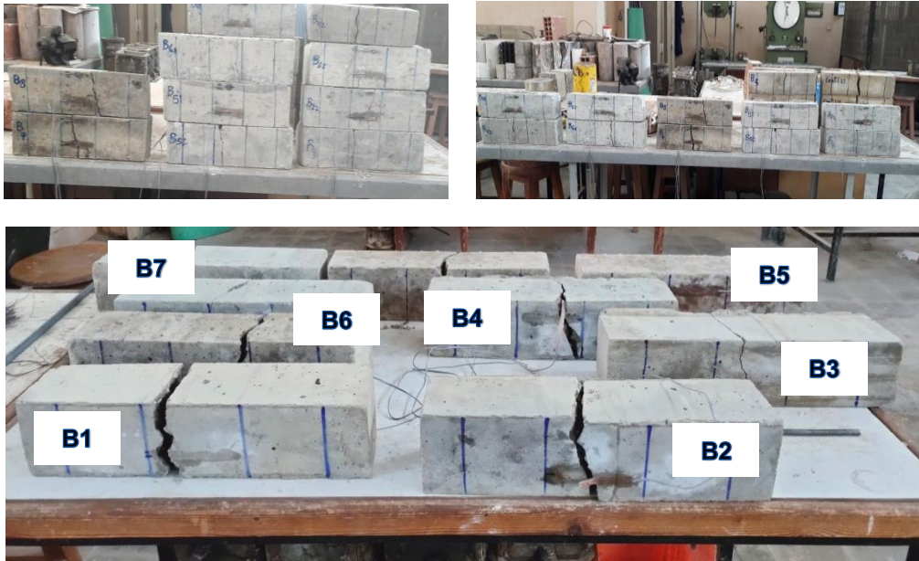
Fig. 9: The crack patterns of tested specimens containing different nano particles
