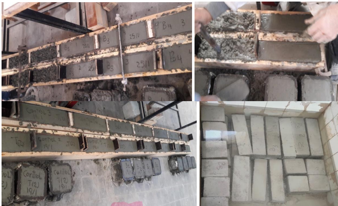
Fig. 2: The tested specimens during casting and curing
