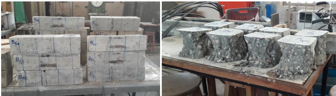
Fig. 4: Failure mode of tested specimens containing different Nano particles
