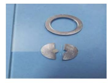
Figure 1: Split mold for disc sample preparation
