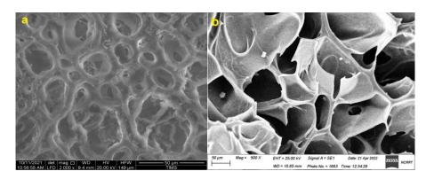
Fig. 6. SEM micrographs of a) Gel-MA(M1) hydrogel and b) Gel-MA/rGO composite hydrogel.
