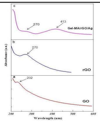
Fig. 3. UV-vis spectra of a) GO, b) rGO and c) Gel-MA/rGO/Ag composite.
