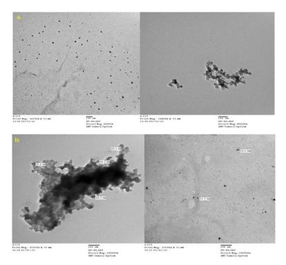
Fig. 7. TEM images of a) rGO and b) Gel-MA/rGO/Ag composite.
