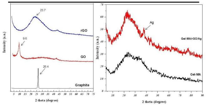
Fig. 4. XRD spectra of a) Graphite, GO and rGO b) Gel-MA hydrogel and Gel-MA/rGO/Ag composite.
