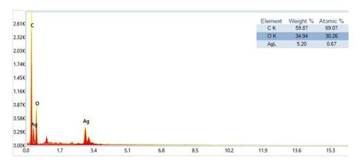
Fig. 8. EDX of Gel-MA/rGO/Ag composite.
