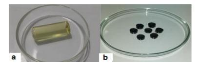
Fig. 1. Hydrogels (a) Gel-MA (M1) in cylindrical form and (b) Irradiated Gel-MA/rGO composite hydrogel discs.
