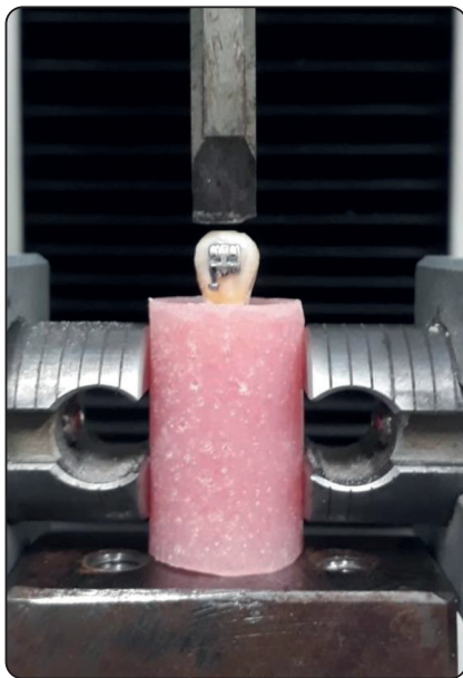
Fig. (2) A tooth embedded in an acrylic block attached to universal testing machine for shear bond strength testing.
