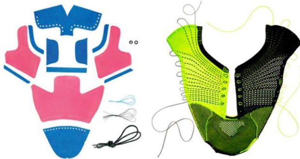
Fig. 2. Components of a traditional shoe upper (left) and a Fly knit upper (right).
