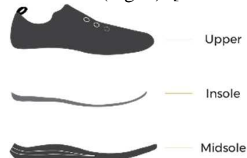
Fig. 1. Main footwear components [Ozdemir, 2020].
