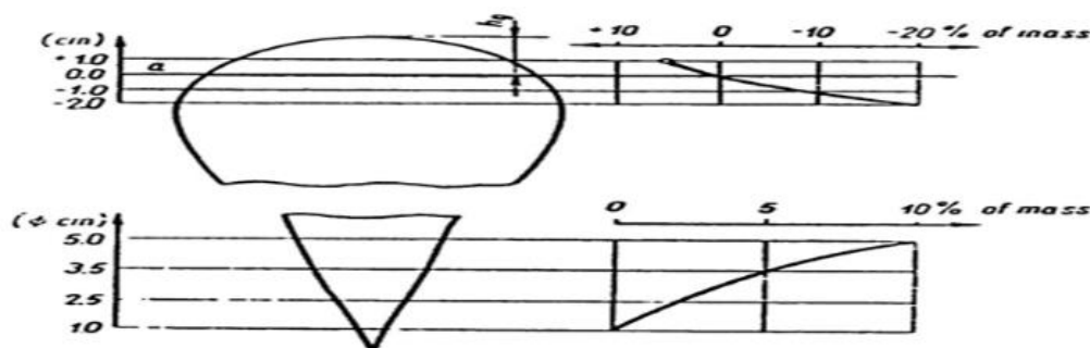
Fig. 1. Critical section of sugar beet cutting.
