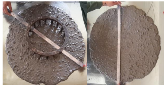
Fig. 2: J-Ring tests & Slump flow
