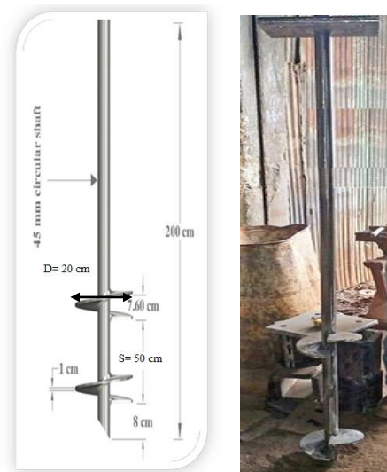
Figure (3): Test Helical Pile Geometry, Dimensions and Shape.
