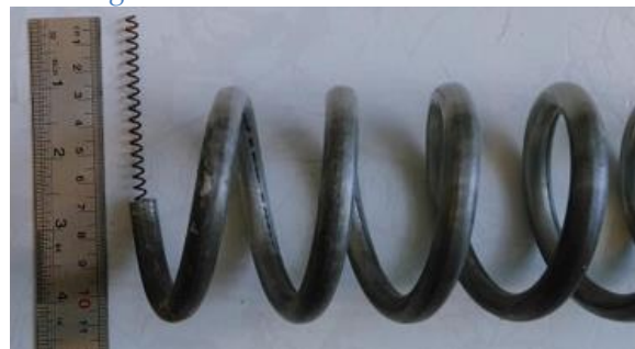
Fig. 7. Spring helical wire as a turbulator in HTHXs [85].
