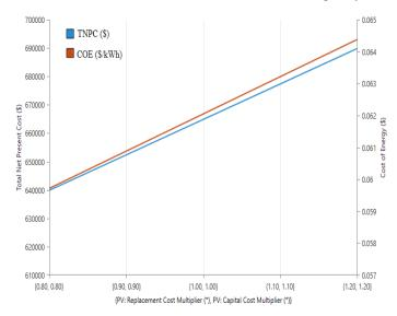
Fig. 11: Sensitivity analysis for PV cost variations on TNPC and COE of the proposed system.
