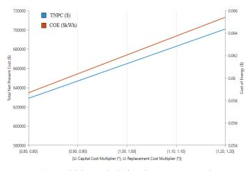
Fig. 12: Sensitivity analysis for Li-Ion Battery Bank cost variations on TNPC and COE of the proposed system.
