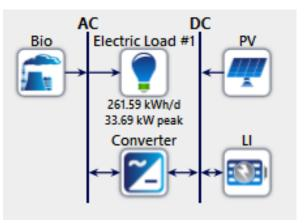
Fig. 7: The schematic diagram of the proposed system.
