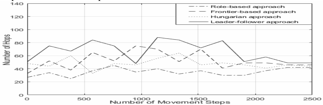
Figure10 Number of steps versus total hop counts in the case of 10 robot for complex map
