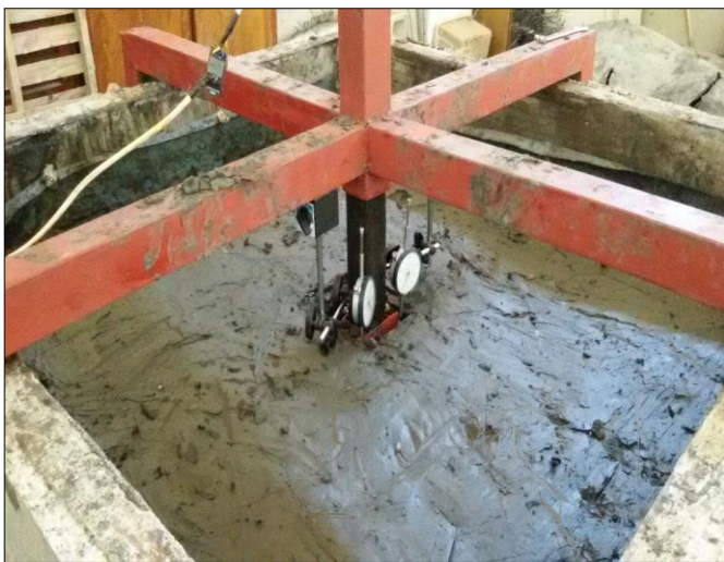
Photo 5 Soil settlement after loading
