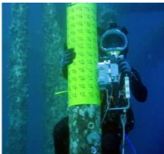
Figure 10: Divers during reading inspection with PEC probe and yellow template for the properly positioning
