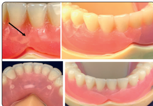
Fig. (5) Fracture Pattern in a) midline in PEKK reinforced OD, b & c) CoCr reinforced OD, d) FRC reinforced OD
