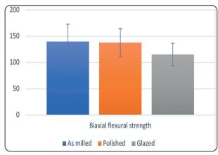
Fig. (2): Bar chart showing mean and standard deviation values (error bars) of biaxial flexural strength for different groups.
