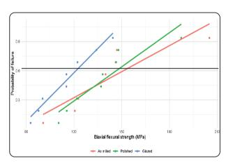
Fig. (3) Probability of failure plot of biaxial flexural strength data.
