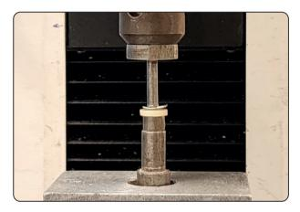
Fig. (1): Biaxial flexural strength test.
