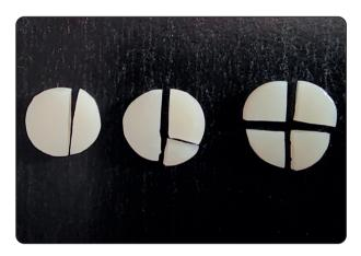
Fig. (4) Different modes of failure according to number of fractured fragments.
