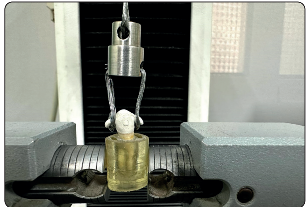
Fig. (1) Application of Pull off test
