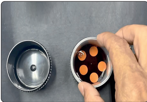
Fig.(4) Samples submerged in bubble-free liquid in dipping jar.
