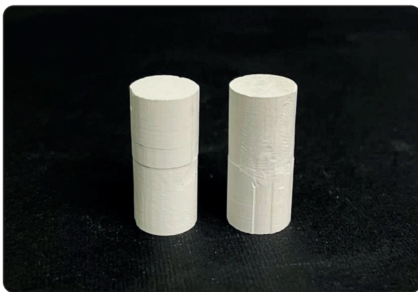
Fig. (1) Monolithic Zirconia blocks milled from zirconia blank
