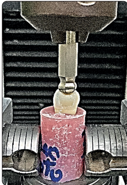
Fig. (2) Static load application perpendicular to long axis of the tooth.
