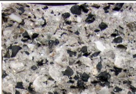
Fig. (9) The Rubber distribution in concrete mixture [N. Oikonomou and S. Mavridou, 2009].
