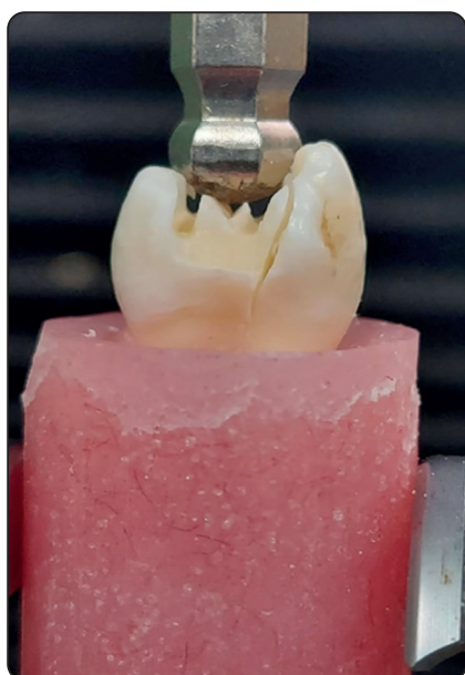
Fig. (1) Showing crack propagation in the premolar prepared with the truss access cavity.
