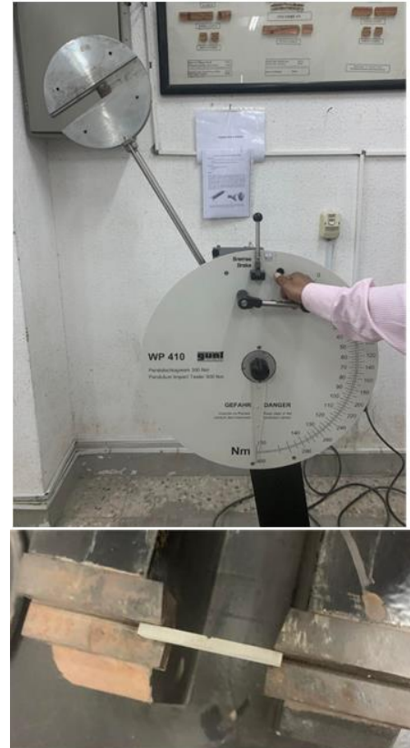
FIGURE 3. Impact test machine and sample setup
