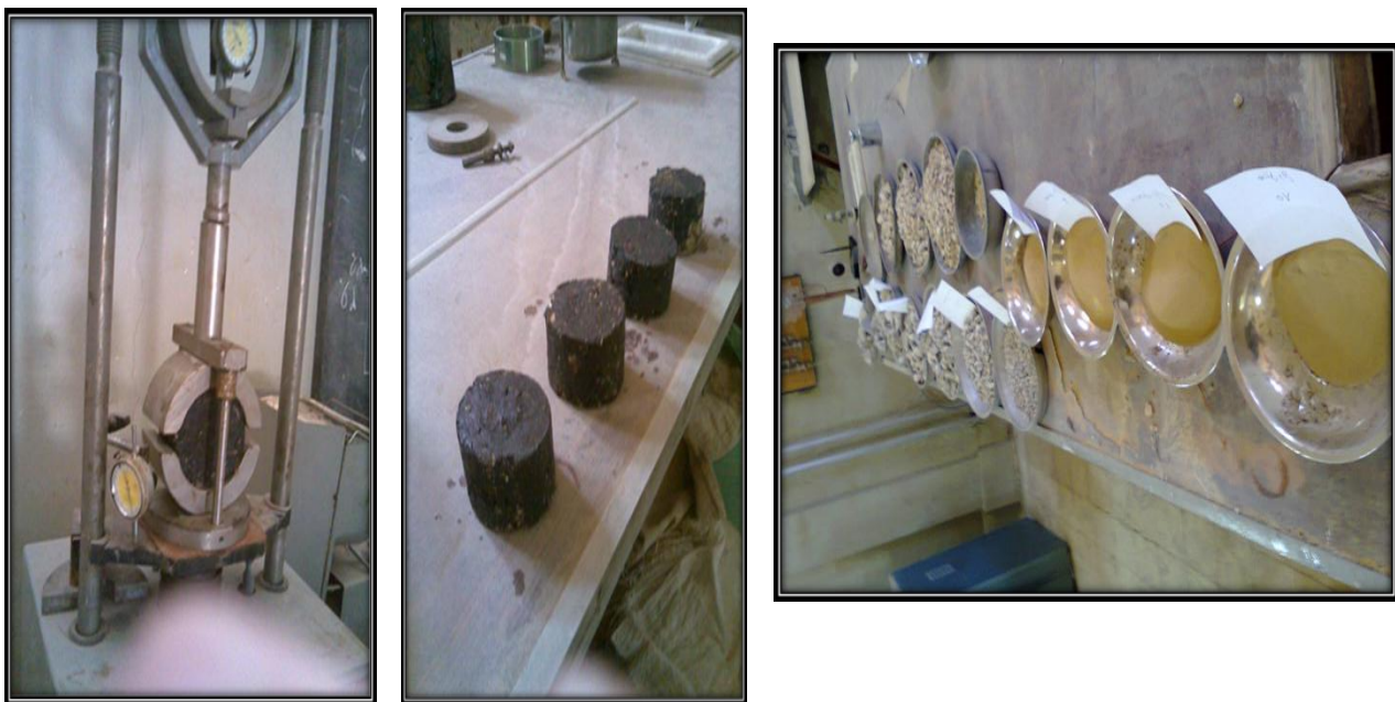
Figure 3: Marshall testing for asphalt concrete mixtures.
