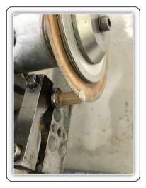
FIG (1) Isomet disc cutting ceramic disc
