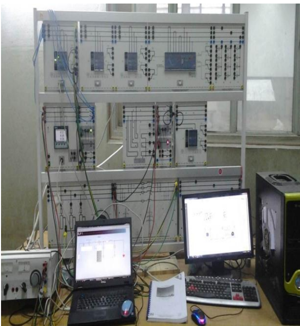
Fig.(7) Lab setup for physical relay test
