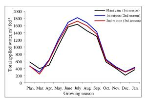
**Fig. 1.** Average monthly irrigation requirement for sugarcane crop at 100% IR
