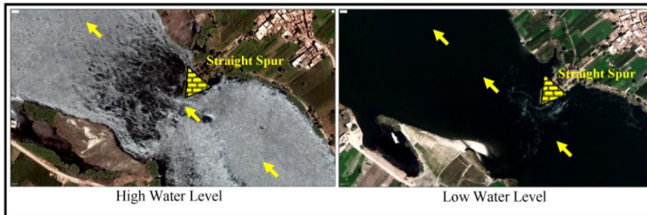
Figure 12: The Impact of Spur Dikes in Creating Extreme Water Vortices as a Result of Their Location at the Curvature Center
