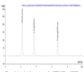
Figure 4: A typical chromatogram for MET, LIN and EMP standard drug.
