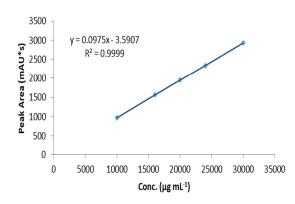
Figure 9: Calibration curve of Metformin using Agilent 1200 with DAD 269 nm.
