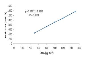
Figure 11: Calibration curve of Empagliflozin using Agilent 1200 with DAD 269 nm.
