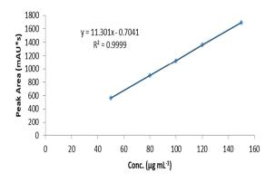
Figure 10: Calibration curve of Linagliptin using Agilent 1200 with DAD 269 nm.
