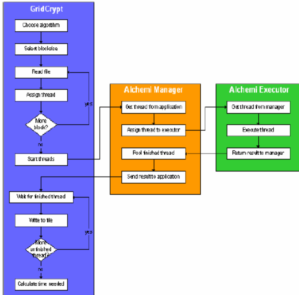
Fig. 3. GridCryptoGraphy flow of process.
