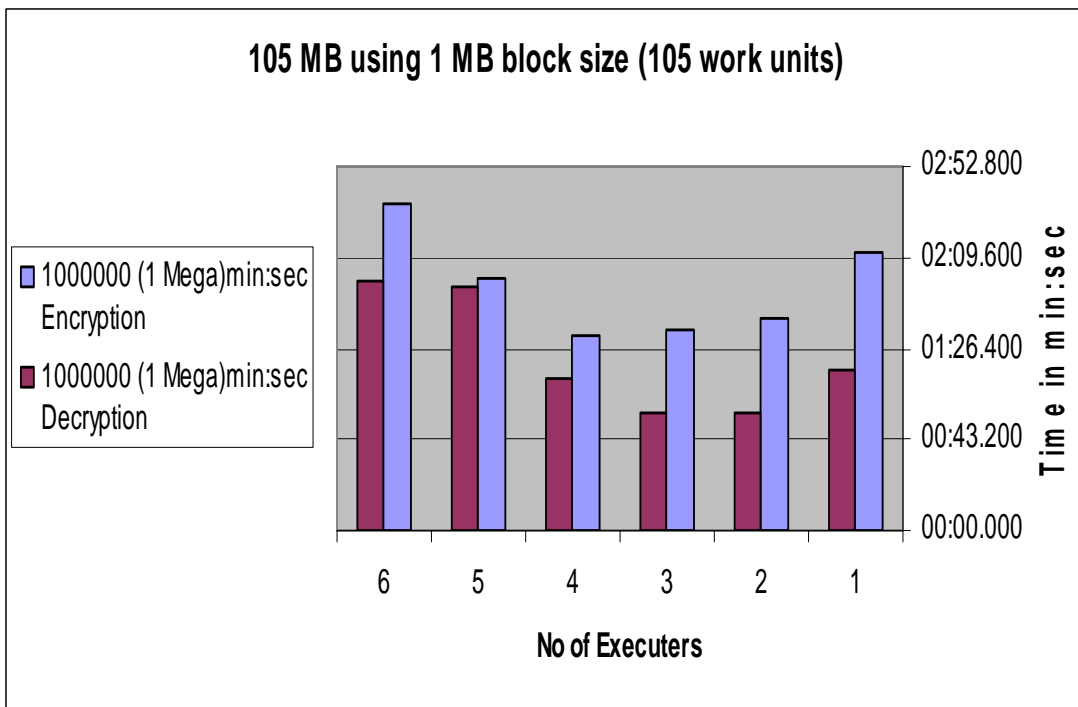
Fig.10. Result graph of (104858112 bytes) file size with 1 Mega block sizes.
