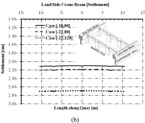
Figure 14: Vertical settlement of crane beams; (a) Sea side crane beam, (b) Land side crane beam.
