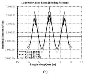
Figure 15: Bending moment of crane beams; (a) Sea side crane beam, (b) Land side crane beam.
