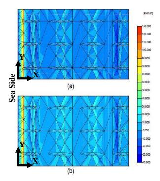
Figure 17: Bending moment in X direction for deck slab; (a) Case (-22, 80), (b) Case (-22, 120).
