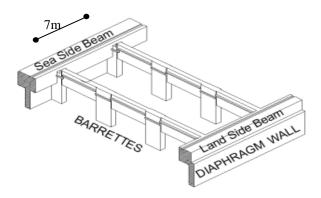
Figure 4: Quay wall beams alignment.
