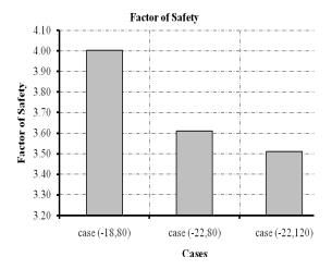
Figure 18:  $\varphi$  – c reduction factor of safety for three cases.
