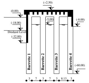
Figure 3: Quay wall cross section.
