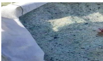
Figure 2. Glass powder utilized in concrete mixtures
