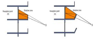
Figure 11 the increasing of shadow zone in balcony by inclining balcony parapet [Source: H.H.El Dien, 2005]
