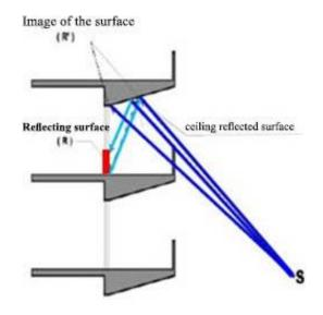
Figure 10 the effect of balcony ceiling form on reception surface of back wall [Source: H.H.El Dien, 2004, by researcher]
