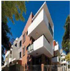
Figure 6 Deep balconies with solid handrails protect from outdoor noise
