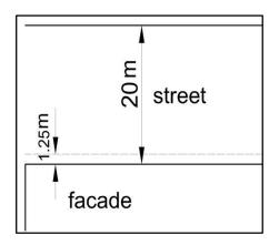
**Figure 20 - limits of a balcony depth on façade surface** [Source: by researcher, Egyptian construction code, 2009]
