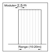
**Figure 18 - limits of façade width and dividing module** [Source: by researcher, Egyptian construction code, 2009]
