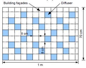
Figure 15 An arrangement of diffusers repeated along façade surface [Source: Picaut, 2010]
