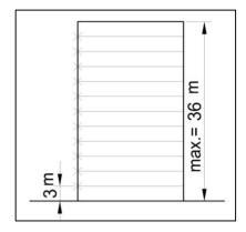
Figure 17 – limits of one floor height and total façade height
