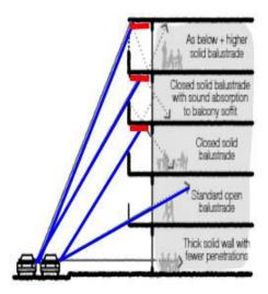
Figure 4 balcony soffits lined with acoustic panels as absorbers
