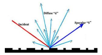
Figure 1 specular and diffuse reflection from façade surface [Source: M.R.Ismail, 2005, by researcher]
