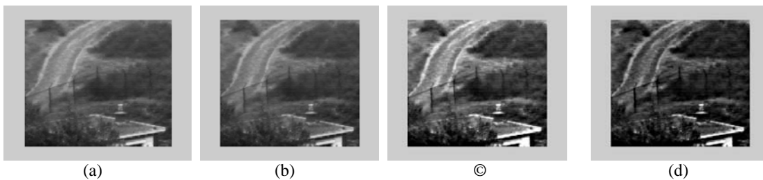
Fig.8. An example of thermal images associated with FPN after applying non-uniformity correction algorithm. (a) Original image, (b) Temporal HPF, (c) Homomorph filter at c=10 , (d) Homomorph filter at c=2 .
