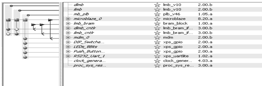
Fig. 20 Xilinx Platform Studio - system assembly view
