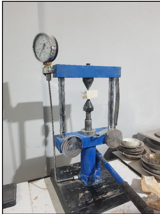
Fig. 9. An experimental setup for PL test on irregular lump specimen. The PL device model: ELE- International Inc. PL tester supplied with load frame for applying loads up to 55 KN.
