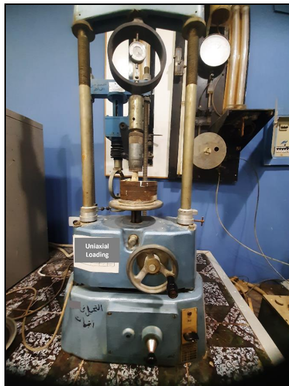
Fig. 5. An experimental setup for UCS test. The device model: ELE-international Inc. for UCS tester supplied with load frame 4 speed 50KN, Proving Ring, 28 KN, Dial Gauge, 0.01x 25 mm and plain platens.
