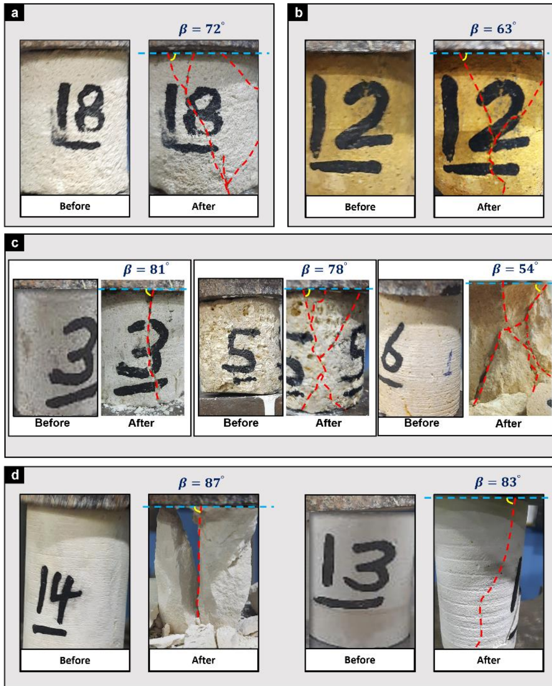
Fig. 8. The observed failure modes and angles in the UCS test (a) Miocene, (b) Oligocene, (c) Upper Eocene, and (d) Middle Eocene. Note: beta ( \beta ) refers to failure angle of the fractured plane.
