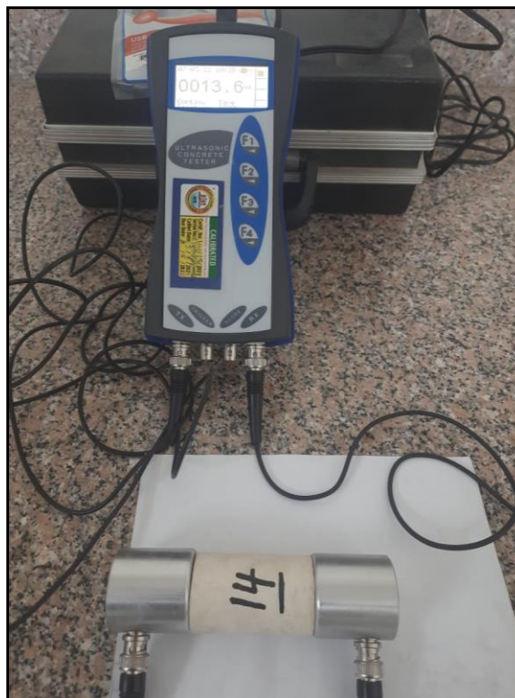
Fig. 11. Performing the UPV test on a known length of an oven-dried core sample. The UPV device model: Matest (C369N) Ultrasonic pulse velocity tester.
