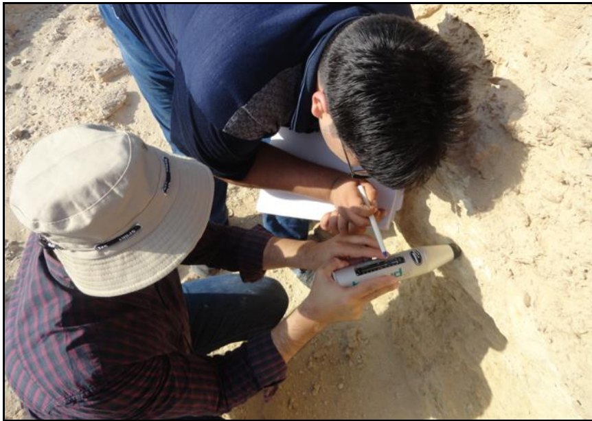
Fig. 10. SH testing on Upper Eocene rock surface. SH testing on Upper Eocene rock surface. The SH device model: Proceq N-type Schmidt hammer.
