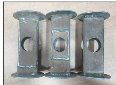
Figure 7. welding parts (Final specimen).
