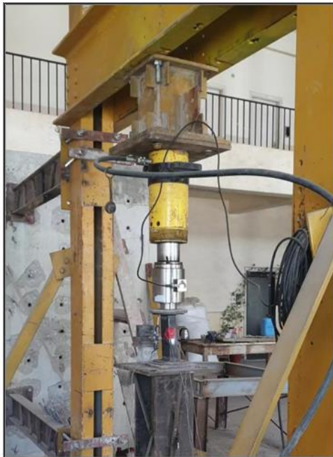
Figure 8. Specimen ends connection.
