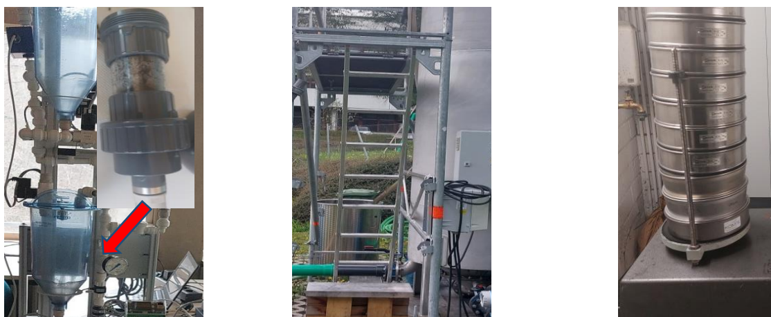
Fig. 1: A) Continuous Lab-scale GAC-Plant: used for the treatment of model wastewater and for finding related kinetics B) Continuous Large-scale GAC plant: used for application of the treatment technology in real wastewater C) Multi sieves apparatus: utilized for particle size distribution.
